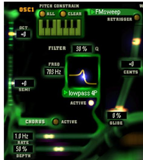
The signal coming into the oscillators from the gate generator first has its pitch detected, no doubt using technology Antares initially developed for AutoTune. The detected pitch is not necessarily the pitch that will come out of kantos, though. First, there is a "pitch constrain" keyboard that can be used to indicate the scale kantos must obey for each oscillator (and, yes, you can set different scales for the two oscillators).
