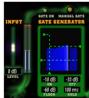
There is also a manual gate that continuously holds the gate open, for example to make it easier to program sounds.
