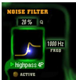
In addition to the two oscillators, kantos provides a noise generator. Like the oscillators, the noise generator features its own resonant filter, which can be enabled or not as needed.
