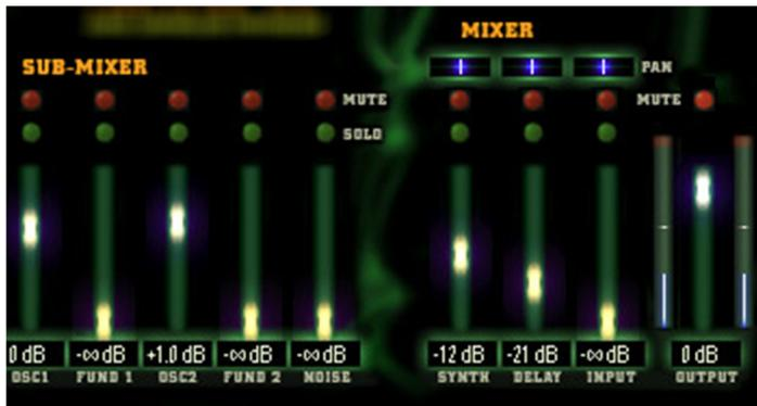
A sub-mixer mixes together the basic signal components. In addition to the articulated outputs of the two oscillators and noise generator, kantos provides the option to mix in some of the fundamental signal from each oscillator. If used, this mixes in a pure sine wave of the fundamental frequency detected by kantos pitch detection circuitry, as modified by any tuning and pitch constraint settings, thus reinforcing the basic pitch, for
