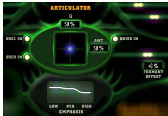
sounds kantos makes, but the articulator is what sets kantos apart from other synths. Its job is to apply harmonic content and formant characteristics from the input signal to the sounds generated within kantos (i.e. by the two oscillators and the noise generator).
