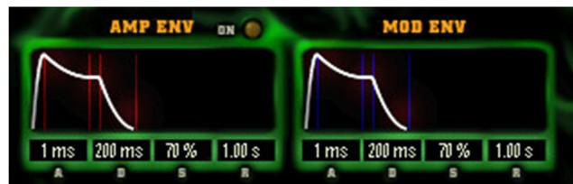
The mod envelope is only available for modulation routing purposes, and will have no effect unless it is routed to some modulation destination.
