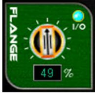
The Flange module provides a simplified flanger, where the only flanging-specific control provided is a flanging depth percentage control. Its effect can range from subtle, for example making a heavily distorted part somewhat less harsh, to lending a bit of motion to a part, to creating a phasey-type sound. Of course, it can also be enabled or disabled via an I/O switch.
