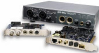
The **Sync Daughter Card** is used for synchronizing with external gear such as video equipment, master clocks, and other DAWs. It includes Word Clock in and out, SMPTE Sync in and out, and MTC (MIDI Time Code) out.
