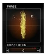
To the right of the peak, perceived loudness, and RMS meters are two meters aimed at monitoring stereo field information. A phase scope is up on top, with a phase correlation meter underneath.
