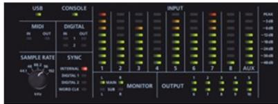
The front panel of the unit provides a sample rate selector, supporting rates of 44.1, 48, 88.2, 96, and 192 kHz. It also provides a wide range of LED-based indicators, including 8-segment input meters, and a sync mode (internal, two digital modes, and word clock) indicator, and MIDI activity meter, among others.
