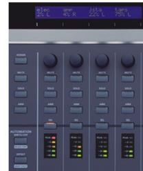
Just to the left of the fader banks, opposite the Mute/Solo/Arm controls are global Mute/Solo/Arm controls. A control assignment button opposite the data adjustment knobs is used for toggling between controls.
