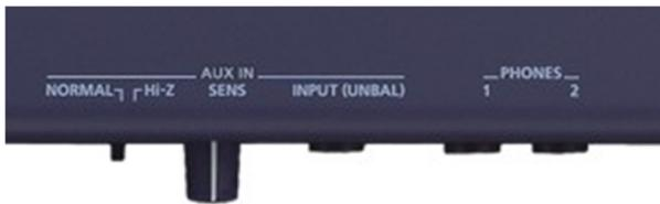
Last, but not least, down on the front right edge of the VS-700C are two quarter-inch headphone jacks plus an unbalanced input that can be switched between line level and Hi-Z (guitar) level for the self-recording musician. There is also an input sensitivity control for fine-tuning the level of the input.
