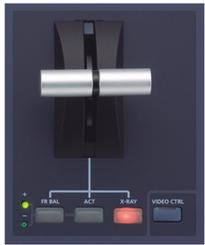
To the left of the surround panner is a multifunction T-bar for surround front/rear balance, controlling SONAR's X-Ray facility (allows plug-ins to become transparent to easily access multiple plug-ins without closing or shuffling them around), or controlling other ACT parameters, as well as for video hardware control.
