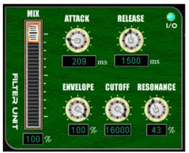
decrease in amplitude. There is also a Mix slider on the Filter Unit to control how much of the incoming signal is passed through the filter, and an I/O switch enables or disables the filter module.
