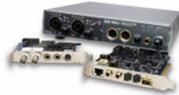
The **Sync Daughter Card** is used for synchronizing with external gear such as video equipment, master clocks, and other DAWs. It includes Word Clock in and out, SMPTE Sync in and out, and MTC (MIDI Time Code) out.
